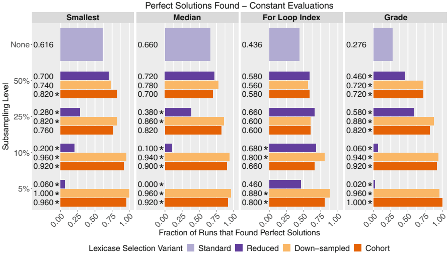
Fig. 1.1 Problem-solving success after 30,000,000 evaluations. Bars show the fraction of replicates that found a perfect solution. An asterisk (*) to the left of a bar denotes a significant difference compared to the standard lexicase results (using a Holm–Bonferroni correction for multiple comparisons). Results for standard lexicase (light purple) consist of 250 replicates per problem, while results for reduced lexicase (dark purple), down-sampled lexicase (yellow), and cohort lexicase (orange) consist of 50 replicates for each configuration
